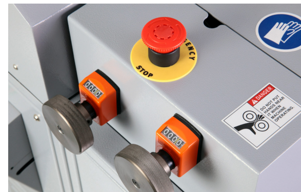
The Auto Gap prevents excess coating from smearing. The roller gap dials can be adjusted in 0.1mm increments.
