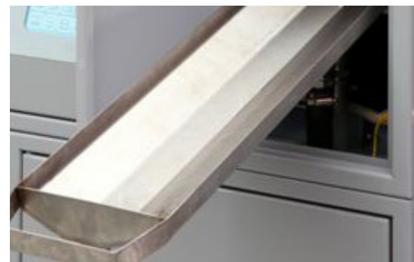
Easy and clean UV oil drip tray removal
