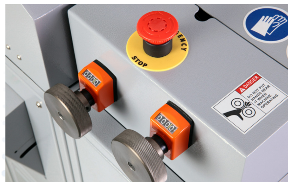
Simple to adjust coating roller gap dials by 0.1 mm
