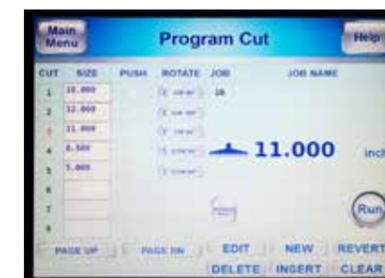
After each cut is completed, the touchscreen control panel will prompt you in which direction to rotate the stack to prevent cutting errors.
