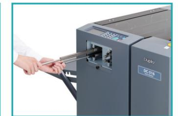
New creasing module includes a dual creasing tool with the capability to perform positive or negative patterns
