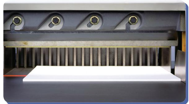
**Simple knife changes** are conveniently made from the front of the machine rather than the side.
