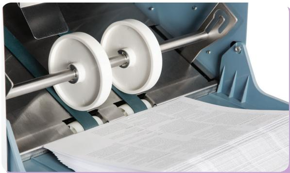
Delivery roller **automatically sets paper size**. Two tray positions are available for enhanced stacking.
